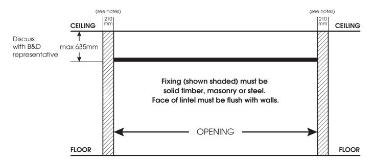
**NOTES:** Measurements shown allow for: Minimum standard overlap - 50mm
