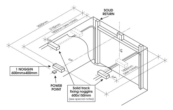
**NOTES:** Doors higher than 2230mm will require two additional fixings at 2400mm.
