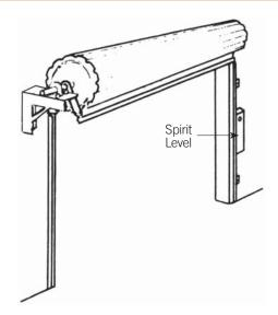
Position guides true and plumb at each side of the opening. Allowing 3-4mm of working clearance between the door and the inside of each guide, mark, drill and fix both guides. Use the 10mm (5/16") coach screws and washers supplied (with suitable plastic plugs for masonry application or other fixings to ensure satisfactory attachment. (Note: Welding of guides to steelwork is usually not recommended).
