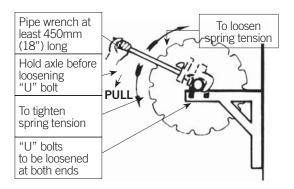
**WARNING:** Hold Axle before loosening "U" bolts. **IMPORTANT:** Do not attempt to loosen "U" bolts before securing firm hold on Axle with Pipe Wrench (Stillson). Do not use files or similar brittle steel tools such as Tommy Bars.
