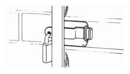
With door fully closed check that bolt slides through guide. Adjust hole if necessary.
