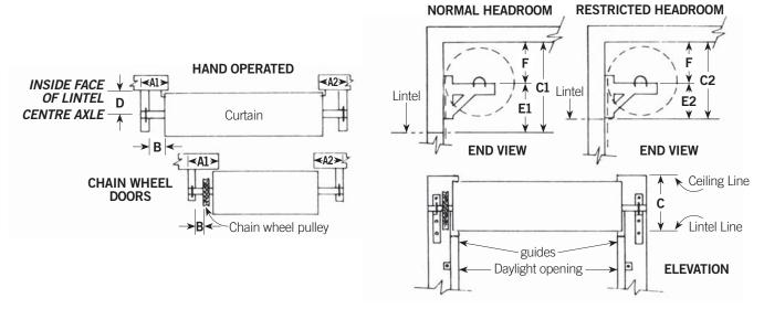
**DOOR SIZE – Width:** The door curtain should be 100mm (see Dimension Panel) wider than the opening. However, a wider than normal door can be fitted by allowing the door to overlap further on each side, providing the additional sideroom is available.
